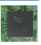
The DR Processor reduces uneven coloring, allowing documents to be scanned as images that are more suitable for OCR (Optical Character Recognition).
